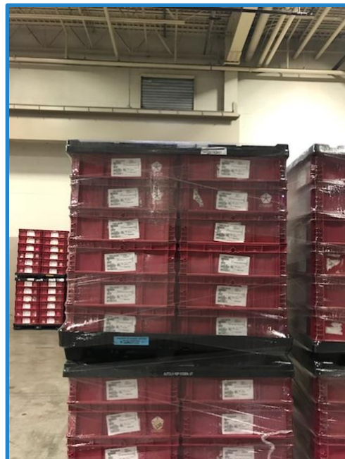
FIGURE 10: EXAMPLE OF A PROPERLY STRETCH WRAPPED PALLET LOAD
